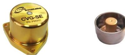
The oscillations in the resonator are generated and detected by piezo-electric actuators, which are attached to the base of the resonator. A closed-loop electronic system is used to control the standing wave oscillation in the resonator, and to null the effects of Coriolis forces induced by the rotation of the resonator, providing as output a signal which is proportional to the gyroscope angular rate.
