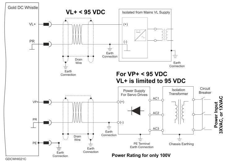
Figure 14: Auxiliary Power Supply Connections Diagram
