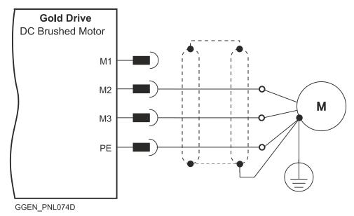
Figure 11: Brushed Motor Power Connection Diagram
