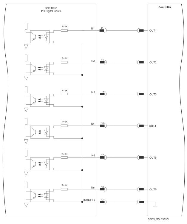
Figure 30: Digital Input TTL Mode Connection Diagram
