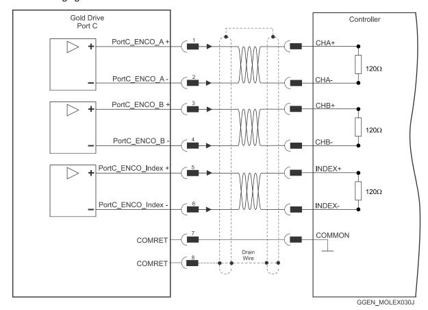
Figure 28: Emulated Encoder Differential Output – Recommended Connection Diagram Note that the user is required to connect a 120  $\Omega$  termination at the end of each differential line.
