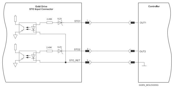
Figure 17: STO Molex Type Input Connection – PLC Source Option
