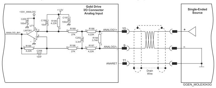
**Figure 29: Differential Analog Input**
