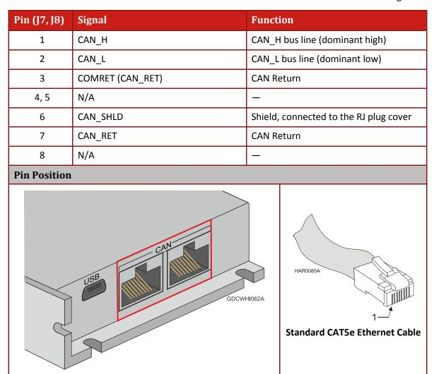
Table 11: CAN In/Out Connectors Pin Assignments
