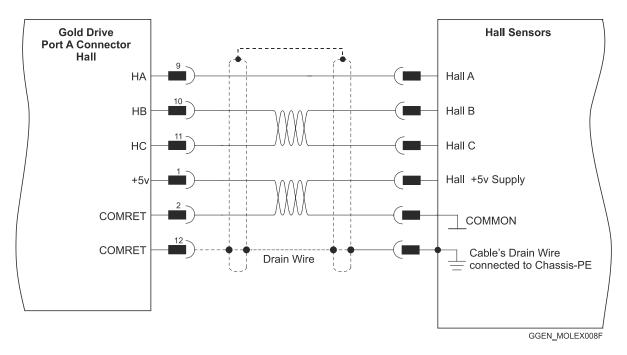
Figure 21: Molex Type Hall Sensors Connection Diagram
