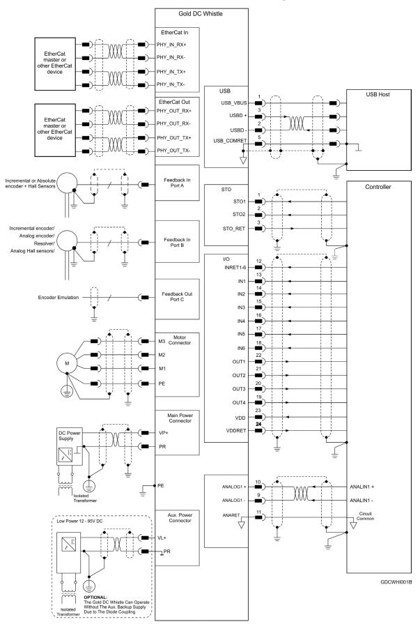
Figure 2: The Gold DC Whistle Connection Diagram – EtherCAT
