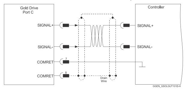
Figure 7: Feedback Port C Cable Assemblies
