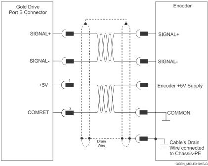
Figure 6: Feedback Port A and B Cable Assemblies
