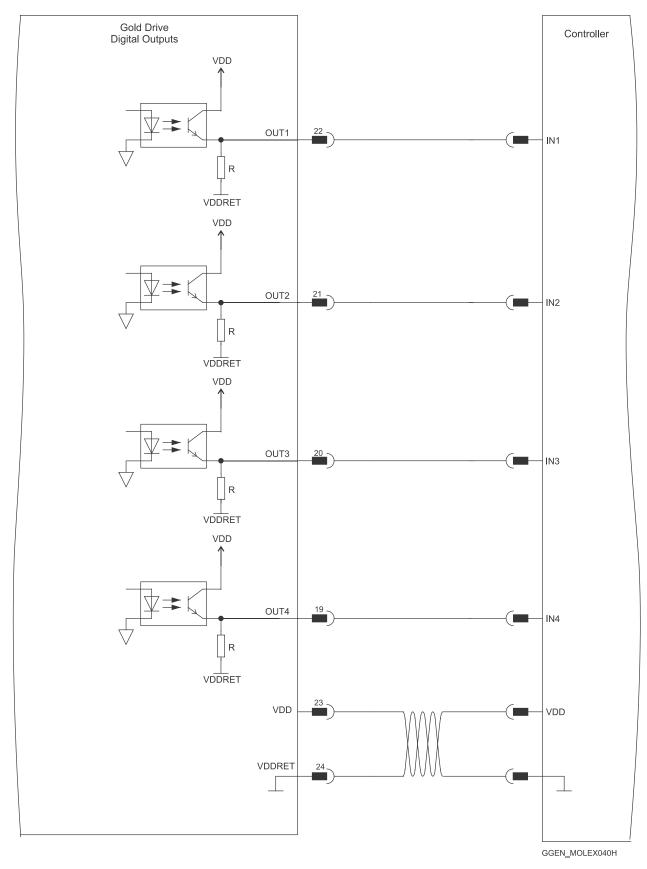
Figure 31: Digital Output Connection Diagram – TTL Option
