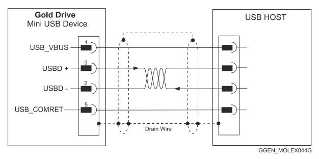
Figure 36: USB Network Diagram
