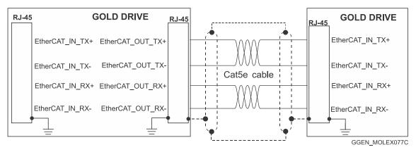
Figure 37: EtherCAT RJ-45 Connections
