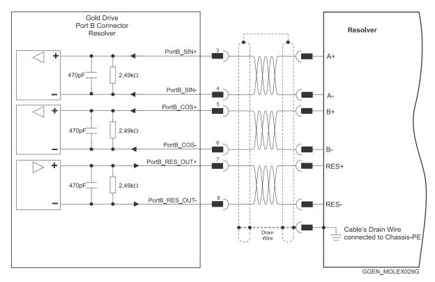
Figure 27: Port B – Resolver Molex Type Connection Diagram
