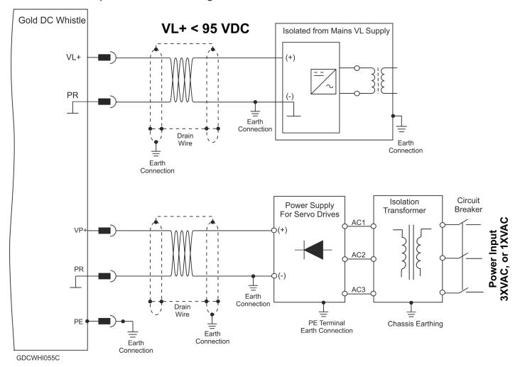
Figure 12: 200 VDC Power Source Connection Diagram
