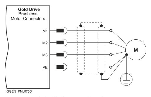
**Figure 10: Brushless Motor Power Connection Diagram**
