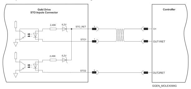
Figure 19: STO Input Connection – Sink Option
