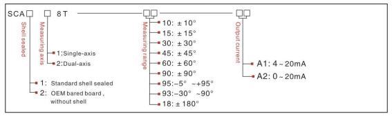
E.g: SCA128T-10-A1: Dual-axis /Standard /±10° Measuring range /4-20mA Output current
