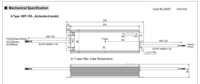
※ IP65 rated. Output voltage and constant current level can be adjusted through internal potentiometer. (Can access by removing the rubber stopper on the case.)
