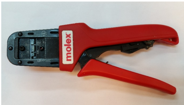
Crimping Tool Molex P/N 63819-1500 Elmo P/N TOOL-P000040
