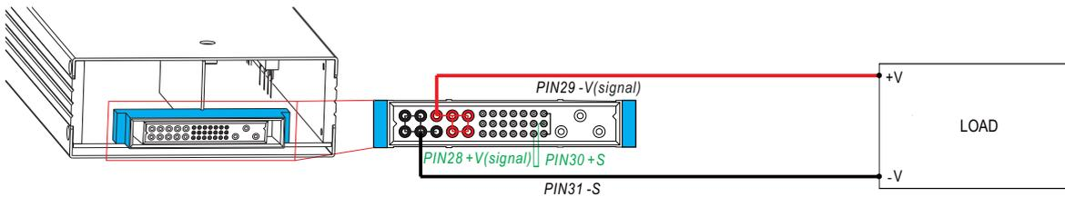
2. Output Voltage Programming (or, PV / remote voltage programming / remote adjust / margin programming / dynamic voltage trim)
