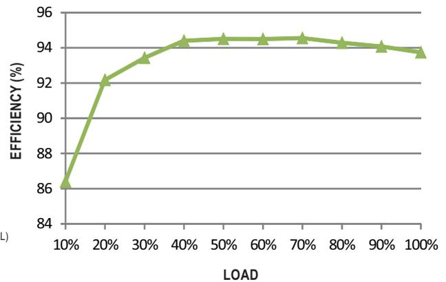
⊙ The curve above is measured at 230VAC.
