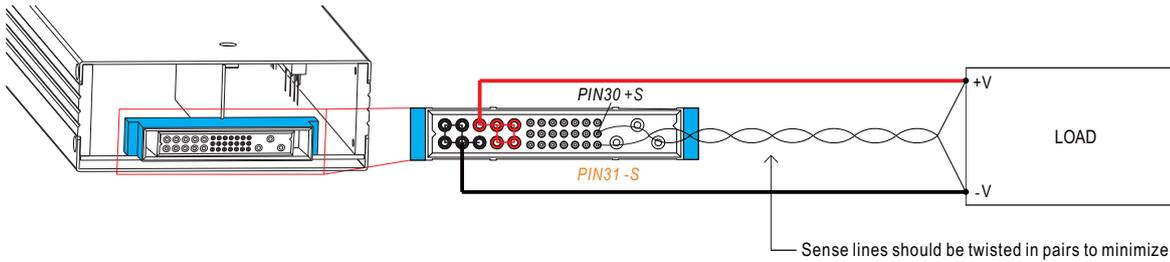
◎ The +S signal should be connected to the positive terminal of the load whereas -S signal to the negative terminal.
