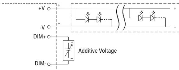
"DO NOT connect "DIM- to -V"
