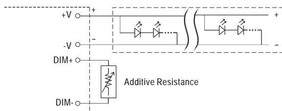
"DO NOT connect "DIM- to -V"
