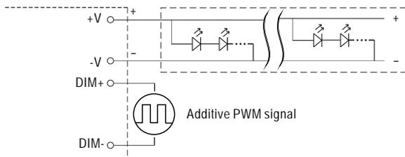
"DO NOT connect "DIM- to -V"
