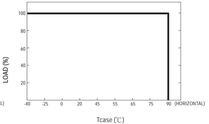
If HVGC-480 operates in Constant Power mode with the rated current, the maximum workable Ta is 55°C (Typ. 230VAC)
