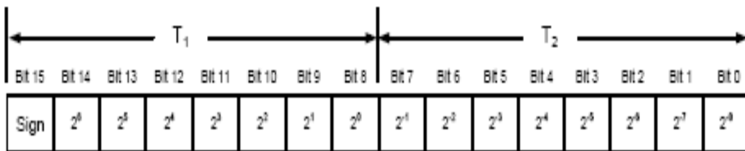
Figure 8-4: Converting temperature data to [°C]
