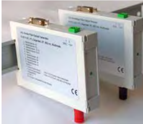
Figure 2. Modules mount on standard 35mm DIN rail
