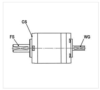
The values for ratios of Harmonic Drive<sup>®</sup> gears refer to the standard input and output arrangement (example 1 in the table below). Other arrangements are possible, and also shown in the table.
