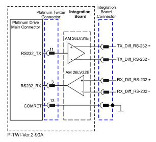
Figure 31: Differential RS232 (RS422) Connection Diagram
