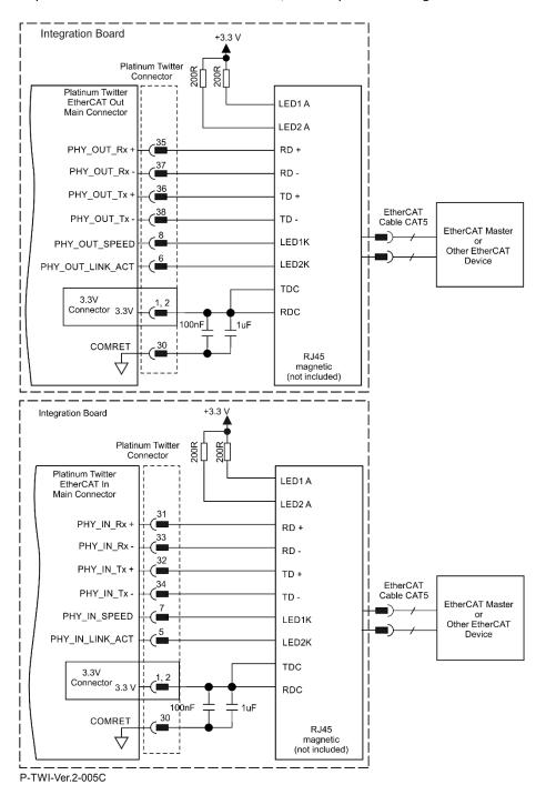
Figure 33: EtherCAT Connection Schematic Diagram
