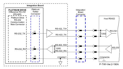
Figure 30: Differential RS-232 Communication Example
