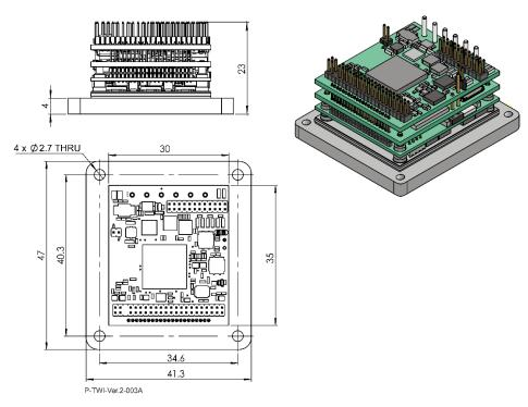
Figure 37: P-Twitter –EtherCAT version with Flat Heatsink
