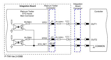
Figure 26: STO Input Connection – PLC (24V Logic)
