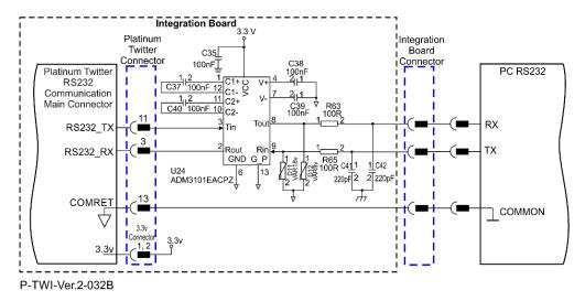
Figure 29: RS232 Connection Diagram
