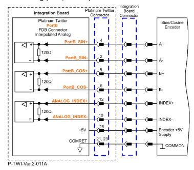
Figure 16: Port B - Interpolated Analog Encoder Connection Diagram
