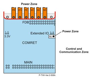
Figure 8: Platinum Twitter EtherCAT Power Conductors PCB layout For more details, refer to section 16.2.2 in the Platinum Safety Drive Manual.
