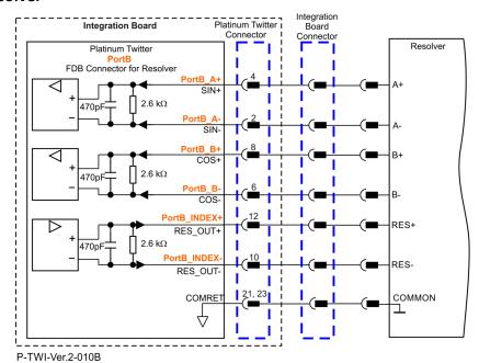
Figure 17: Port B – Resolver Connection Diagram
