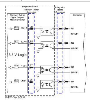
Figure 24: Digital Output 3.3V Logic Mode Connection Diagram
