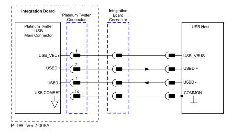
Figure 32: USB Network Diagram
