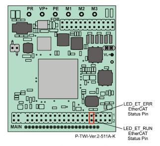
Figure 34: EtherCAT Status Indicator Pin
