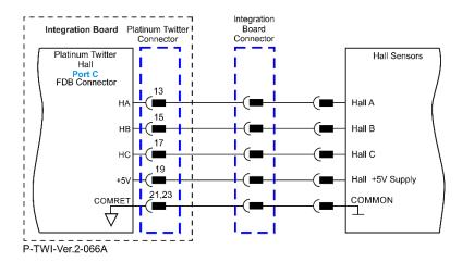
Figure 22: Hall Sensors Connection Diagram
