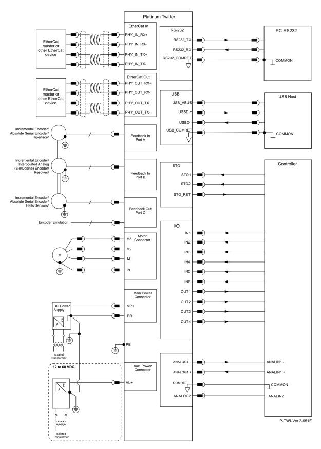
Figure 6: The Platinum Twitter EtherCAT Connection Diagram
