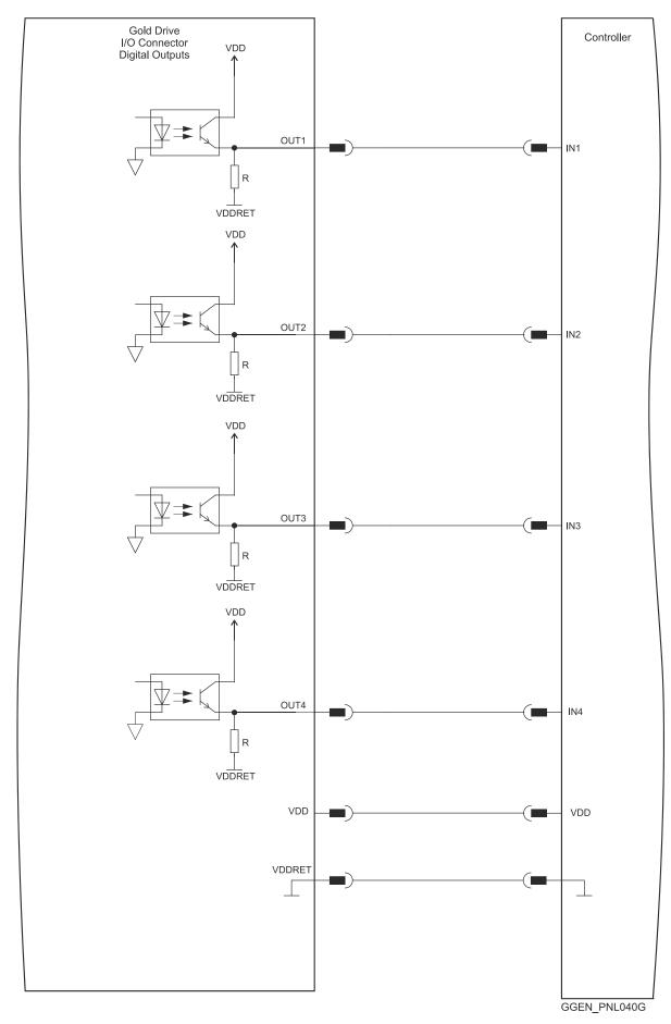
Figure 45: Digital Output Connection Diagram Example – TTL Option
