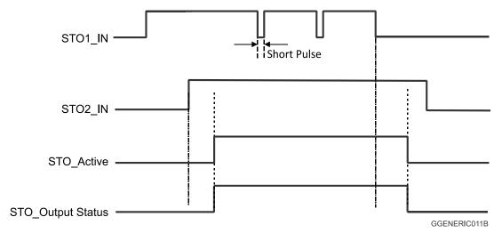
Figure 12: STO Output Status Timing Diagram (Refer to STO Timing)
