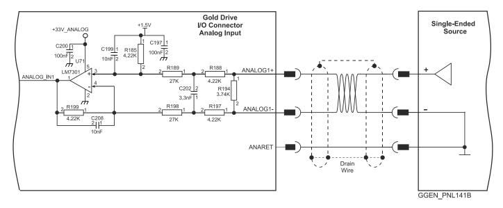
Figure 55: Differential Analog Input for Shrouded Type connector
