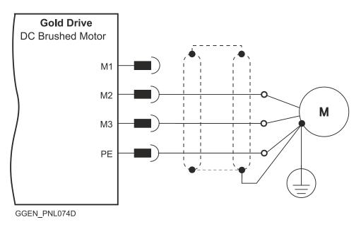
**Figure 4: DC Brushed Motor Power Connection Diagram**
