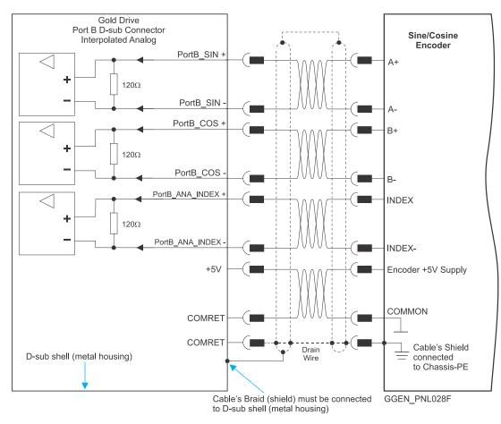
Figure 31: Port B - Interpolated Analog Encoder D-Type Connection Diagram Example
