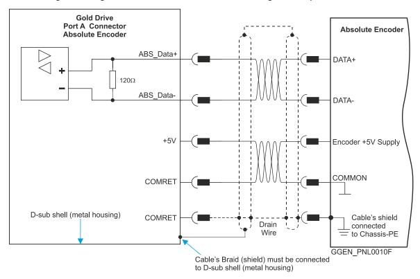
Figure 24: Absolute Serial Encoder – D-Type Connection Diagram Example for Sensors Supporting Data Line Only (NRZ types, e.g., Panasonic / Tamagawa / Sanyo / Nikon)
