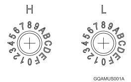
**Figure 60: EtherCAT Address Switches**
