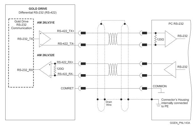
Figure 67: Differential RS-232 RJ-45 Communication Example
