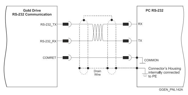
Figure 65: RS-232 RJ-45 Connection Diagram Example
