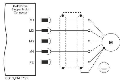
**Figure 5: Stepper Motor Power Connection Diagram**
