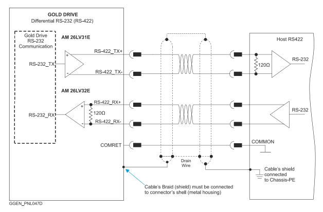
Figure 66: Differential RS-232 D-Type Communication Example
