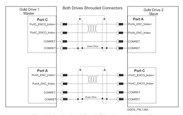
Figure 39: Port C to Port A Shrouded Type Connections Example
