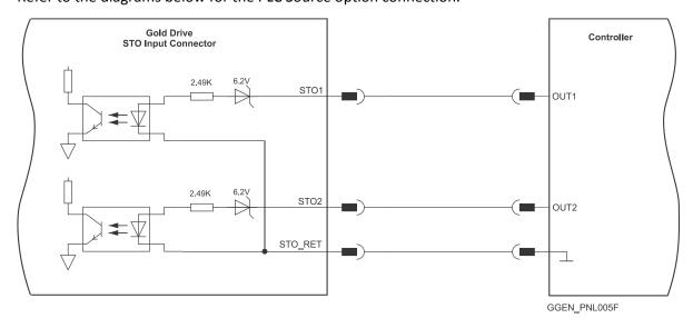
Figure 8: STO Input Connection Example – PLC Source Option
