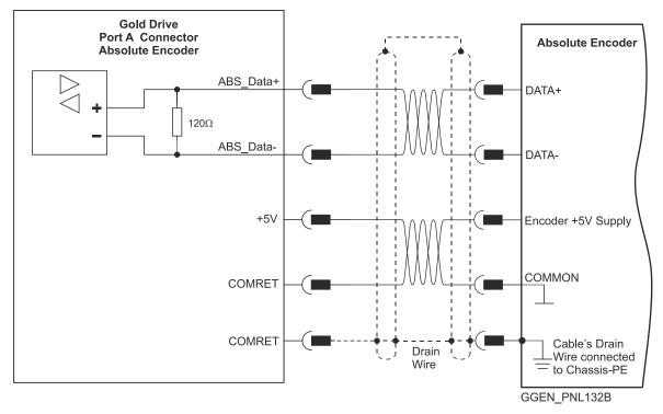
Figure 25: Absolute Serial Encoder – Shrouded Type Connection Diagram Example for Sensors Supporting Data Line Only (NRZ types, e.g., Panasonic / Tamagawa / Sanyo / Nikon)
