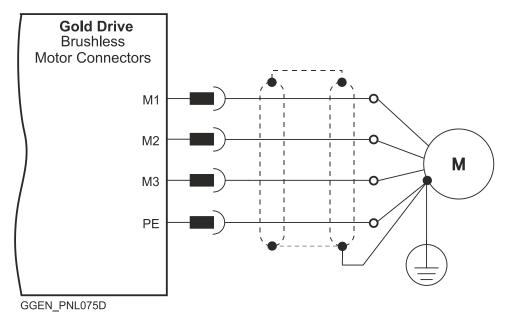
Figure 3: Brushless Motor Power Connection Diagram
