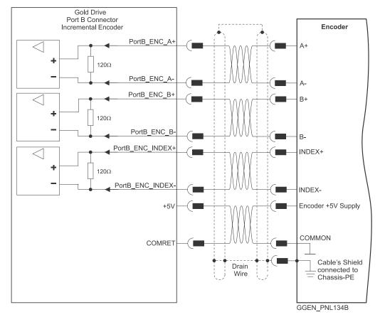
Figure 30: Port B Incremental Encoder Input – Shrouded Type Connection Diagram Example
