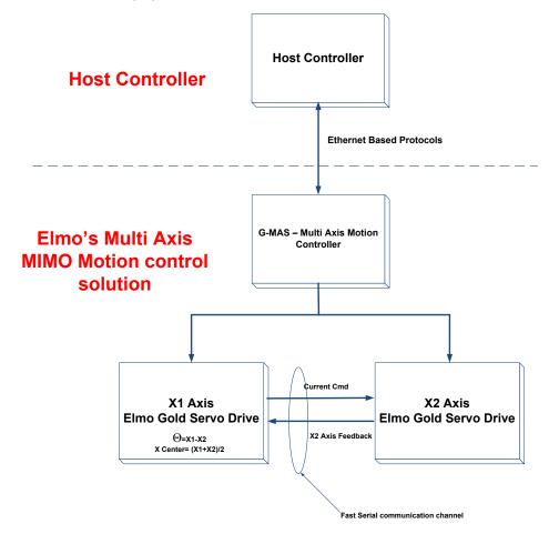
Figure 37: Flexible Gantry system
