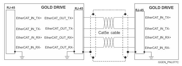
Figure 57: EtherCAT RJ-45 Connections Example
