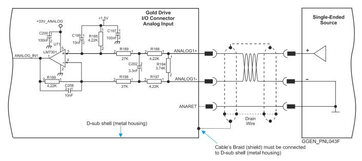
Figure 54: Differential Analog Input for D-Type connector
