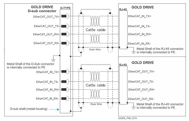
Figure 59: EtherCAT with D-TYPE Connections Example
