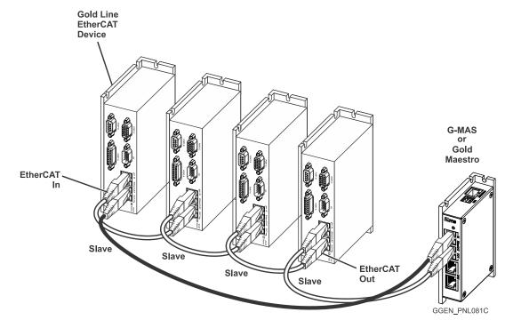
Figure 62: EtherCAT Network with Redundancy
