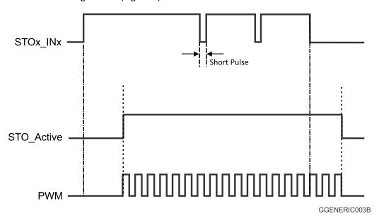
Figure 6: Timing Diagram of short pulses
