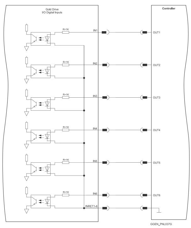
Figure 43: Digital Input TTL Mode Connection Diagram Example
