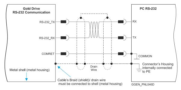
Figure 64: RS-232 D-Type Connection Diagram Example
