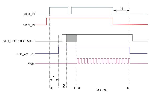
Figure 14: STO Signals Timing Diagram
