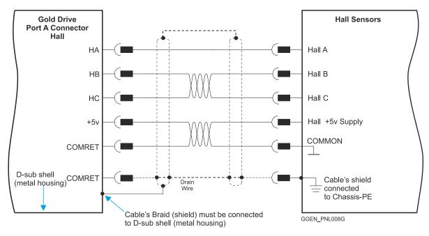
Figure 20: Hall Sensors D-Type Connection Diagram Example
