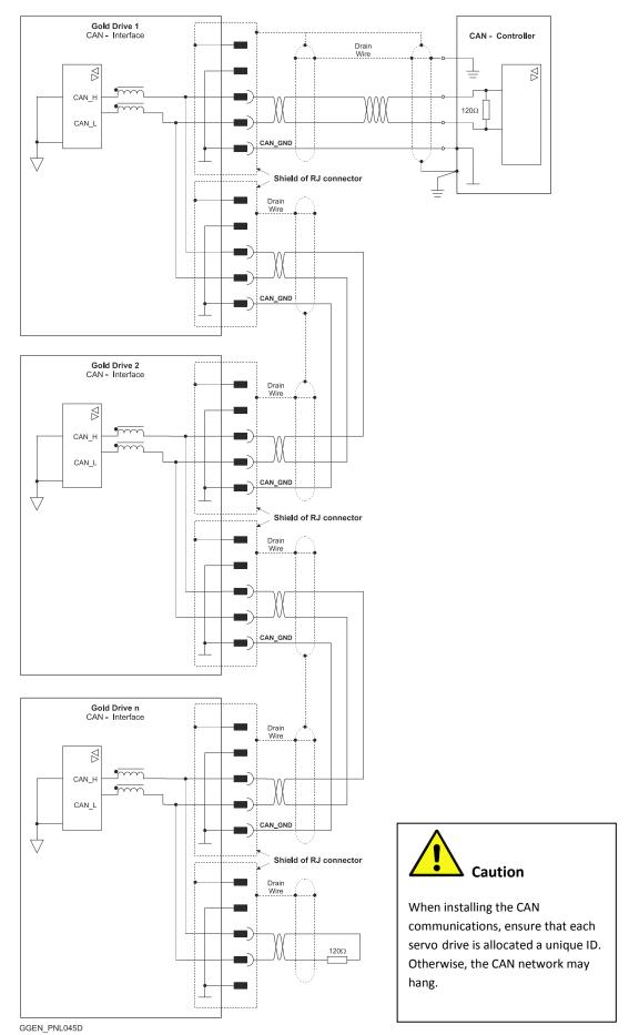
Figure 63: Gold Panel Mounted Servo Drive Connection Diagram Example – CAN
