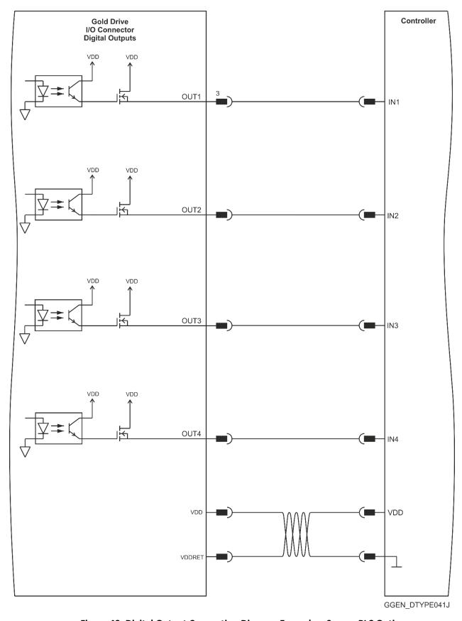
Figure 49: Digital Output Connection Diagram Example – Source PLC Option
