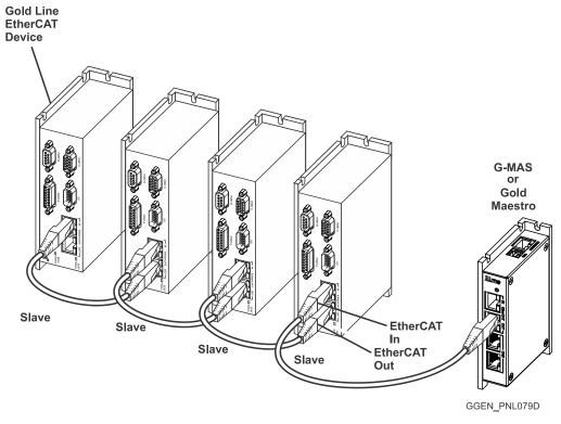
Figure 61: EtherCAT Network with No Redundancy
