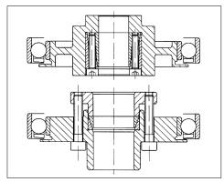
Design examples for Solid Wave Generator with clamping element
