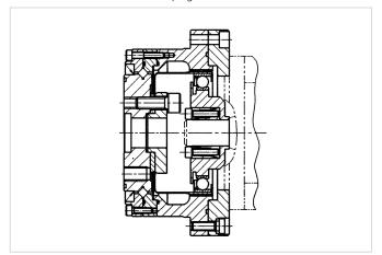
For stepping motor operation and for large motor shaft diameters the use of a solid Wave Generator is recommended. Illustration 50.1 shows the standard version with Oldham coupling and keyway. Illustration 50.2 shows a solid Wave Generator without Oldham coupling. The Wave Generator is attached directly to the motor shaft by means of a clamping element.
