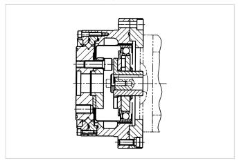
Illustration 50.2 Units with Clamping Element
