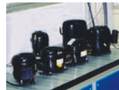
Compressor for Air Conditioner
