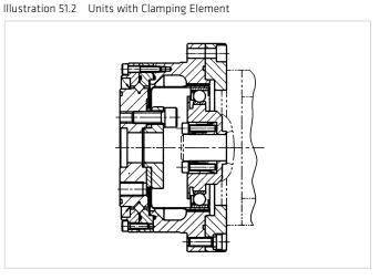
For stepping motor operation and for large motor shaft diameters the use of a solid Wave Generator is recommended. illustration 51.2 shows the standard version with Oldham coupling and keyway. Illustration 51.2 shows a solid Wave Generator without Oldham coupling. The Wave Generator is attached directly to the motor shaft by means of a clamping element.
