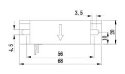
This product is a molded part, the material is PC+PBT, the shape and installation size tolerance is in accordance with GB/T14486-2008 MT6.
