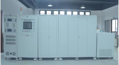
Farad: HY-CHCTSU-300-20KVA-D10kV High Current & High Voltage Test system for Thin film capacitors (purchased in 2021) 1000A ripple high current test system Output bandwidth: 100Hz-2kHz adjustable
