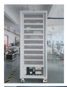
Huawei: HY-CTSSU series AC 0  $\sim$  50.0V adjustable, resolution 0.01V DC 0  $\sim$  2000.0V adjustable, resolution 0.1V Application: Film capacitor characteristic test
