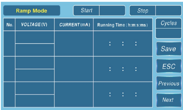
The gradient setting page can set the required voltage, frequency, running time, initial step and end step.
